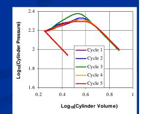
Increasing gasoline input per cycle
