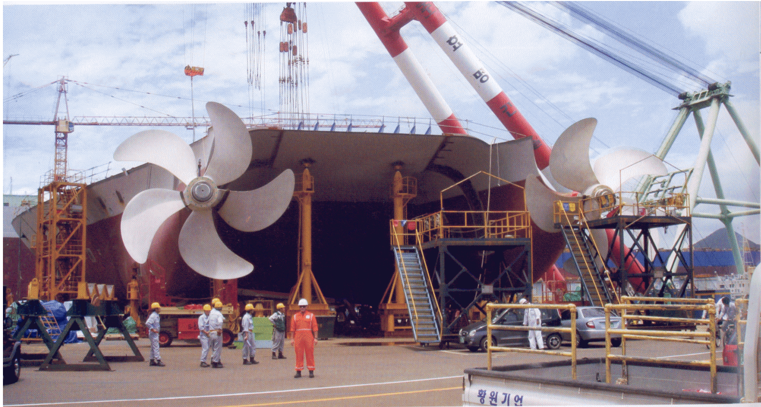
Each propeller on a Q-Flex ship is about 25 feet in diameter and weighs around 80,000 pounds. The ships are powered by twin engines that total 44,000 horsepower.
