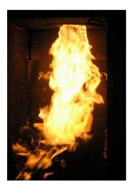
60% NH<sub>3</sub> by Energy 34% NH<sub>3</sub> by Energy in H<sub>2</sub> (15 KW)
