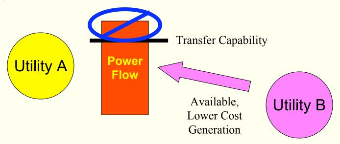
Utility B has cheaper power available, but can't move the power to Utility A because of transmission constraints "between" Utilities A and B (the lines will become congested if Utility B generates additional power)
