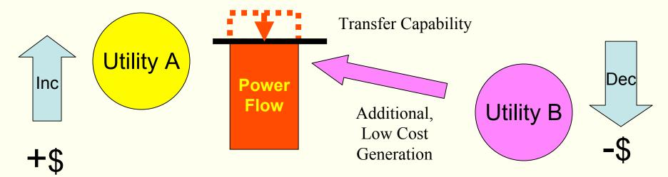
The fee for this service is the difference in cost of increasing generation (or decreasing load) on the "load side" of the constraint less the costs saved by not having to generate (or increase load) on the "supply side" of the constraint. It is economic to do this deal when the savings to Utility A of buying lower cost power from Utility B is less than the cost of the redispatch solution.
