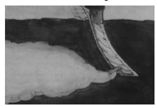
Anhydrous ammonia expands into a gas as it is injected into the soil where it rapidly combines with soil moisture.
