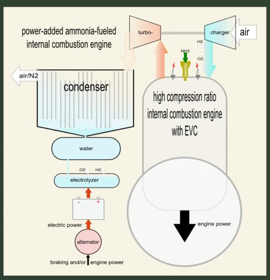
scenario 1: double-punch—vapor+combustion power
