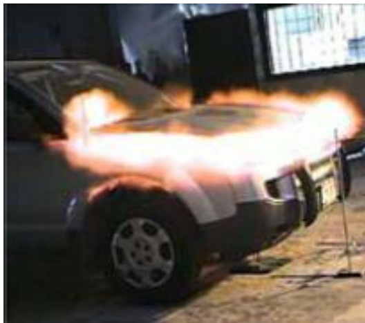
Ignition of engine compartment hydrogen release
