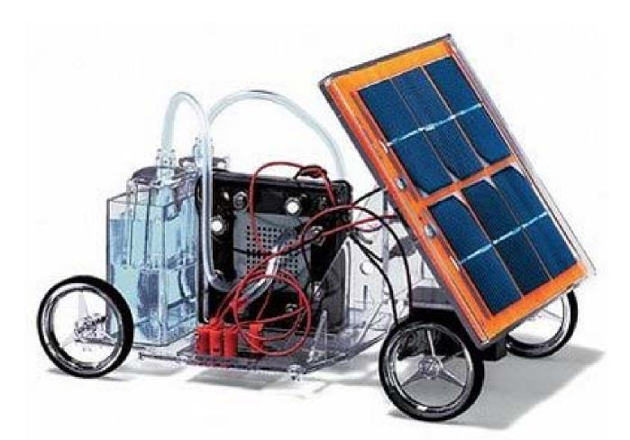
A fuel cell that may be run in electrolytic mode – generating fuel when power is provided.
