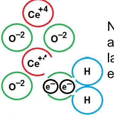
New oxygen vacancy (w/H<sub>2</sub>O) assists with proton conduction, lattice electron assists with electronic conduction.
