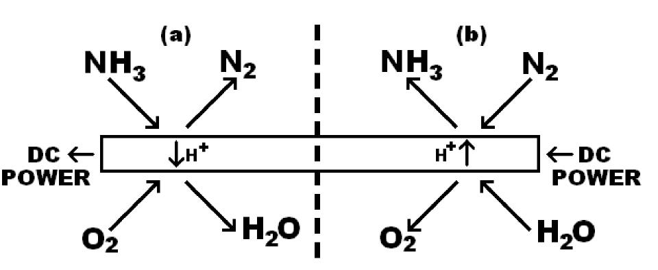
PCC membrane operating in (a) fuel cell and (b) fuel synthesis modes.
