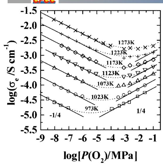
This study observes hole (p-type) conduction at high oxygen partial pressure... and holes are part of the protonic fuel cell process.
