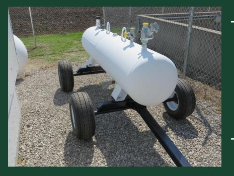
When the collector tank is full, a valve allows the NH3 to flow into the 120 gallon ammonia storage tank.
