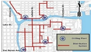
Chicago's district cooling network is one of the largest in the world
